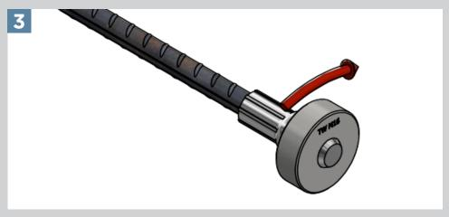
At the end of the PSE thread hand-tighten the TEC coupler with as much force as possible to make sure the coupler is fully engaged.
