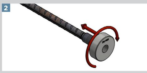
Hand-tighten the TEC End coupler onto TSE coupler.
