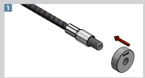
Align the TEC End coupler with PSA-PSC coupler. The PSC Bolt should be fully engaged in the PSA coupler and tightened with an allen key.
