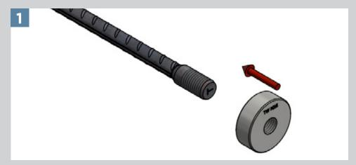
Align the TEC End coupler with TSE coupler.
