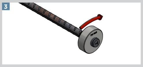
At the end of the TSE thread hand-tighten the TEC coupler with as much force as possible to make sure the coupler is fully engaged.
