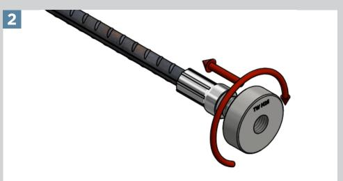
Hand-tighten the TEC End coupler onto PSE coupler.
