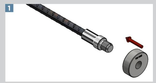
Align the TEC End coupler with PSE coupler.
