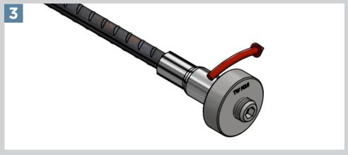
At the end of the PSC thread hand-tighten the TEC coupler with as much force as possible to make sure the coupler is fully engaged.
