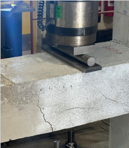
Figure 3 - Application of load to slab / wall test sample
