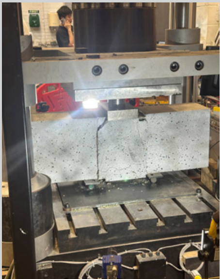
Figure 4 - Longitudinal shear tests
