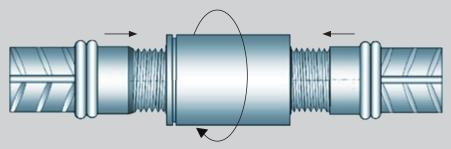
3 Both sections are then screwed together by turning the female coupler. The finished joint tightened with a torque wrench until no further movement and torque requirements of table 2 are met. For correct installation and maximum thread cover both ends should meet in the middle of the female coupler.
