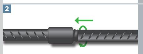
Remove the plastic cap from the coupler. Position and rotate the continuation bar in the coupler.
