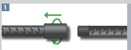
Fix and rotate the coupler to the rear of the thread on the fixed bar and lock tight. The bar end should be central within the coupler.
