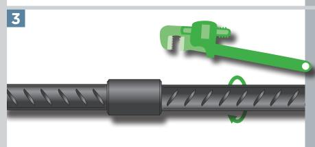
**Tighten the joint** using a wrench on the continuation bar. After tightening there should not be more than 2 - 4 mm of the thread exposed, depending on the diameter of the rebar, to reach the specified torque values given in Table 1.
